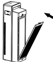
Step 5: Reattached the rear cover of the unit and securely latch into space.
